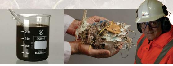
SLF has reduced emissions of sulphur dioxide and oxides of nitrogen by 15% compared to using fossil fuels alone. The most recent alternative is *Climafuel*, a fuel made from household waste that is processed to a tight specification. It reduces landfill and saves fossil fuels for future generations.
